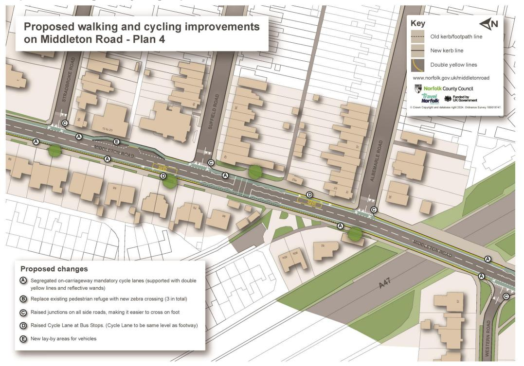
Plan 4 is a drawing of an aerial view of a street map with buildings showing the proposed improvements for walking and cycling on Middleton Road. This drawing shows, from right to left, the section of Middleton Road from the junction with Western Road, heading northwards to the junction with Stradbroke Road.
