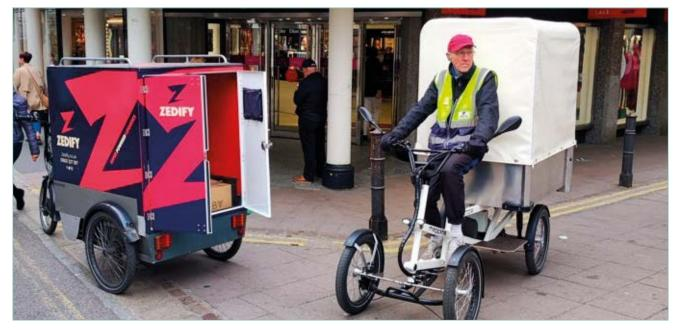
Figure 10: Example of an E-cargo bicycle. Source: Zedify, 2021
